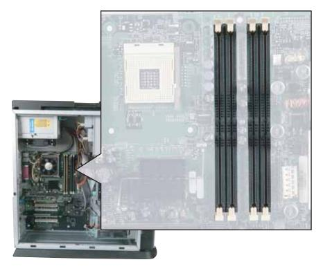
**3** If you are removing a DIMM from the memory module bank, gently pull the plastic tabs away from the sides of the memory module and remove it.
